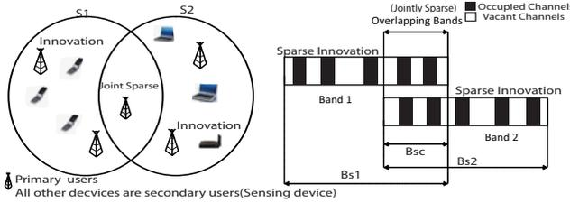
Fig. 2. Schematic of overlapping networks and overlapping spectrum bands
