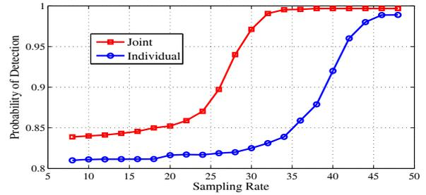
Fig. 5. POD using individual and joint reconstruction in noisy measurements
