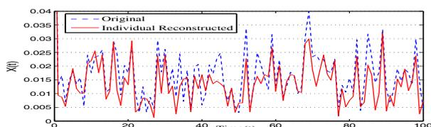
Fig. 10. Original time domain signal and reconstructed signal using individual reconstruction method
