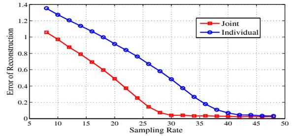
Fig. 6. EOR using individual and joint reconstruction in noisy measurements
