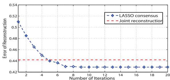
Fig. 9. EOR comparison, For SNR=-5dB, S.R=0.6 and Sparsity=40%
