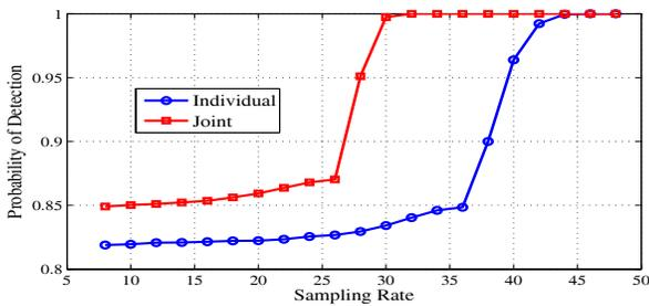
Fig. 3. POD using individual and joint reconstruction
